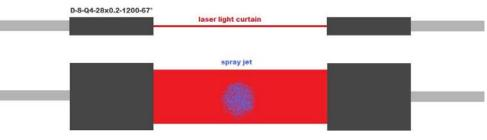
transmitter can be 150mm. At the output of the **A-LAS-CON1-FIO** there is an analogue signal available (0V ... +10V or 4mA ... 20mA) which informs about the amount of spray or density of the spray jet (can be chosen in the software) and furthermore digital signals which informs, whether the amount or density of the spray jet is in tolerance.
