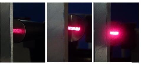
placed outside the Ex – range. The maximum distance between transmitter and receiver frontend is approximately 150mm. The measurement range is about 6mm. As shown in the screen shots the blades can be positioned precisely.
