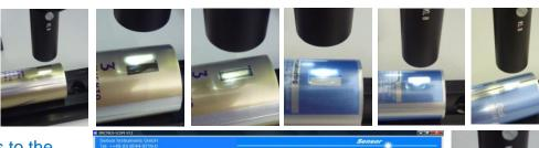
background color as well as to the glue line. At this a color sensor type **SPECTRO-3-FIO-CL** in connection with an optical fiber type **R-S-R2.1-**(6x1)-1200-67° and an optical frontend type **KL-8-R2.1** are used. The distance of the frontend to the color mark is approximately 18mm and the white light spot size is
