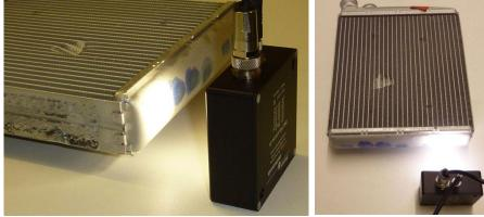
the **SPECTRO3 Scope** Windows® software offers the possibility to put all of the different blue spay marks together into one group, thus a proper recognition of the spray mark is possible.
