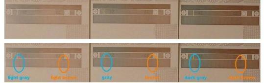
runs out of tolerance. For the tests a color sensor type **SPECTRO-3-FIO-JR** in connection with an optical fiber type **R-S-R2.1-(6x1)-1200-67°** and an optical frontend type **KL-8-R2.1** is used. The distance from the frontend to the paper is approximately 11mm. The white light spot size at this distance is around 4mm x 0.7mm. A proper detection of the gradient in the gray as well as in the brown range of the reference color mark is possible.
