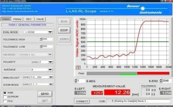
microns and the scan frequency is about 600 Hz. As shown in the screenshots, there is a proper detection of the margin of the respective abrasive belt possible.
