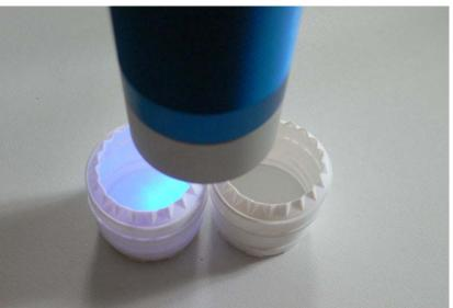
**SPECTRO-3-30-UV** fluorescent color sensor to check, whether the additional seal inside the enclosure head is present or not. Due to the fact, that the additional seal is UV fluorescent, the differentiation is very easy.
