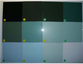
Direct reflection: **SPECTRO-3-50-FCL** is directed perpendicular to the respective glass plate and the direct reflection from the glass plate will be measured. At this the upper surface delivers no information about the glass type, while the reflection on the lower surface of the glass plate informs about the light absorption due to glass.
