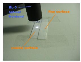
Used sensor: SPECTRO-3-FIO-CL with R-S-A2.0-(2.5)-1200-67° and KL-3-A2.0.
