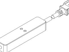
cab-4/USB-... or cab-4/USB-w-... (no picture) (each max. length 5m, outer jacket: PUR)
