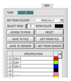
With SAVE TO SENSOR and GET FROM SENSOR the TABLE ATTRIBUTES can now be saved to the sensor and loaded from the sensor.
