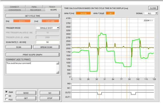
In addition to **CH0**, the signal value **SIG** is transferred in the SCOPE tab.
