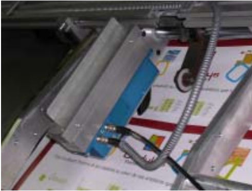
Picture 3 Copy counting at compensating stackers (LCC-80, LCC-80-MA)
