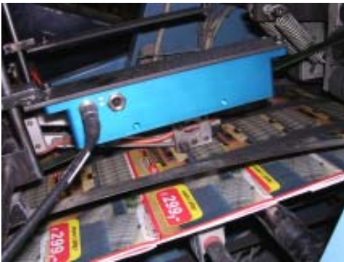
Picture 5 and 6 Copy counting during overhead conveyance (LCC-90, LCC-90-MA)
