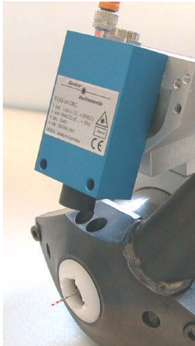
Laser light barrier R-LAS-LR-OBC mounted at drill head
