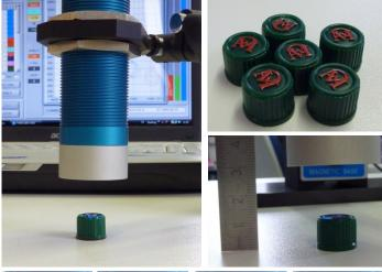
differ, too. The SPECTRO-3-30-UV comes with a detecting range of 12mm at a distance of 20mm; furthermore the sensor
