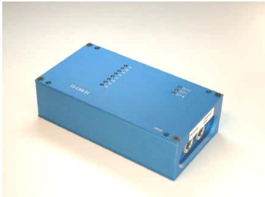
With the SCOPE34 Windows® software the SI-CON34 control unit can be parameterised through the RS232 interface.
