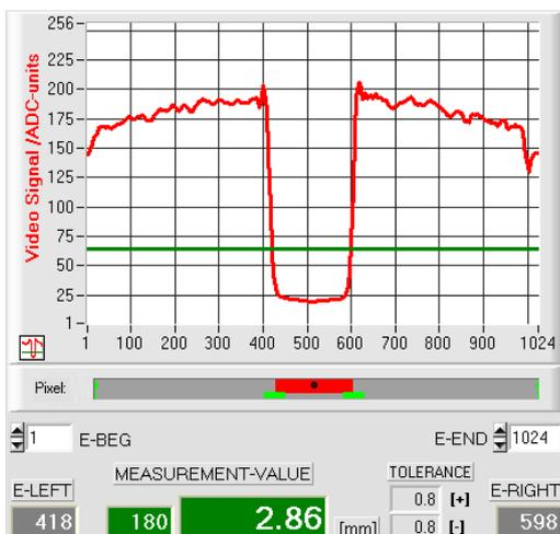
High video threshold, the object appears wider in the "shadow zone". Measured value = 180 pixel. The measured value in µm is calculated from this by multiplying the number of pixels with the respective pixel pitch.
