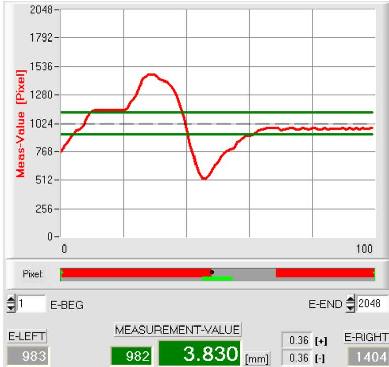
After a click on the RUN button the current measurement value is shown in the graphic display window in "scroll mode". In the form of a red curve the measurement values pass through the graphic display window from the right to the left.
