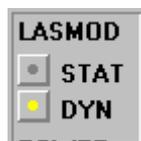
Then the laser operating mode should be set to DYN. In addition DIST must be set in the MEASURE selection field.
