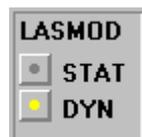
Then the laser operating mode should be set to DYN. In addition DIST must be set in the MEASURE selection field.
