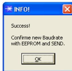
When the new baudrate information has been successfully sent, the sensor operates with the new baudrate. A window will pop up, prompting you to select **EEPROM** and then to press **SEND**. After a hardware reset the new baudrate only will be used when **EEPROM** and **SEND** have been pressed.
