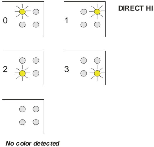
If **DIRECT LO** is activated, the specially digital output is set to LO, while the other 3 are set to HI. If the current color does not correspond with any of the teach-in colors, color C-No = 255 is set, i.e. all digital outputs are set to HIGH (all LED are lighting).
