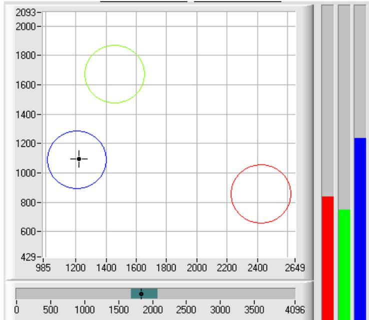
X/Y/INT or s/i/M: A panel opens that shows the taught color spheres and the current color position. For improved representation a three-side view with the graphs X/Y (s/i), X/INT (s/M) and Y/INT (i/M) was chosen.
