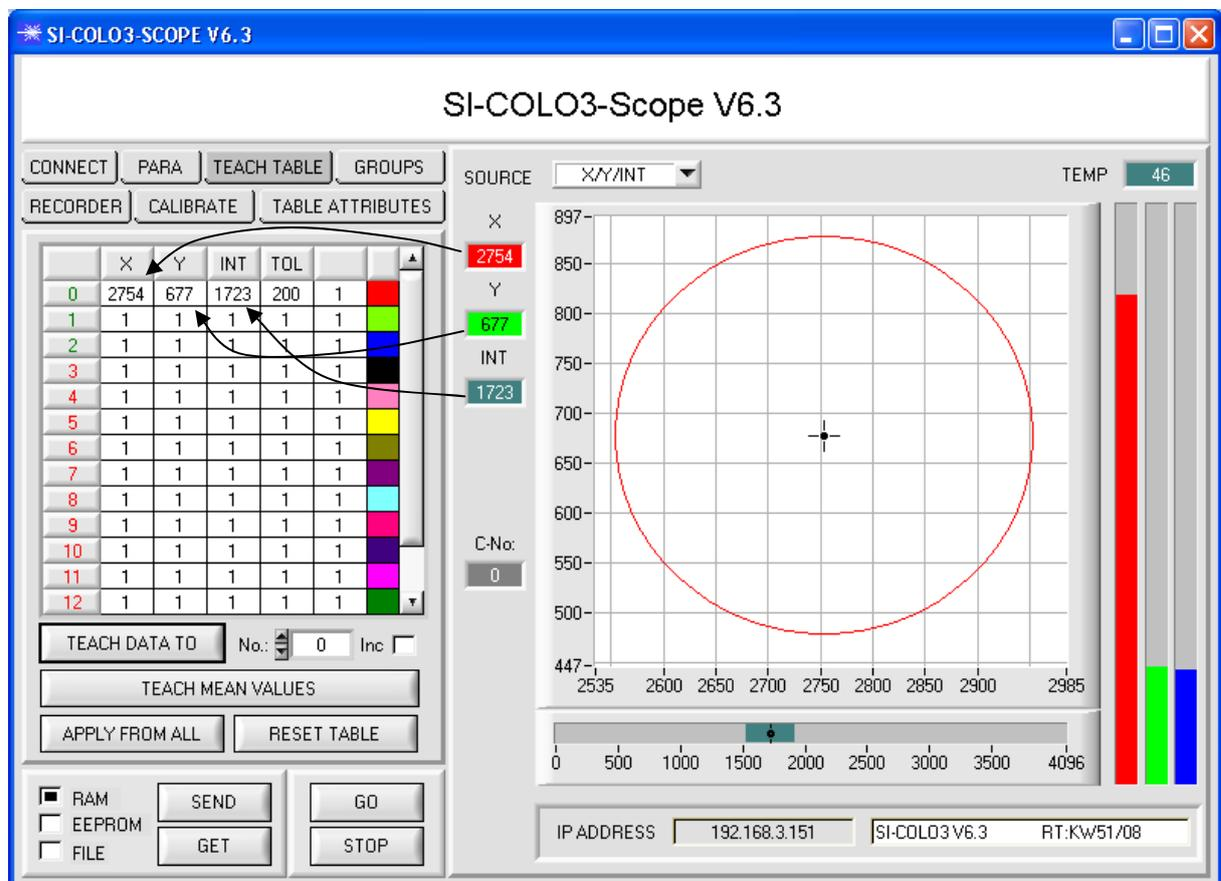
Now press the **SEND** button again to inform the sensor about the taught color. Then activate the **GO** mode again. When the sensor recognises a row vector (color), the corresponding row number is visualised on the software interface under **C-No.:**. A value of 255 means that none of the taught colors were recognised.
