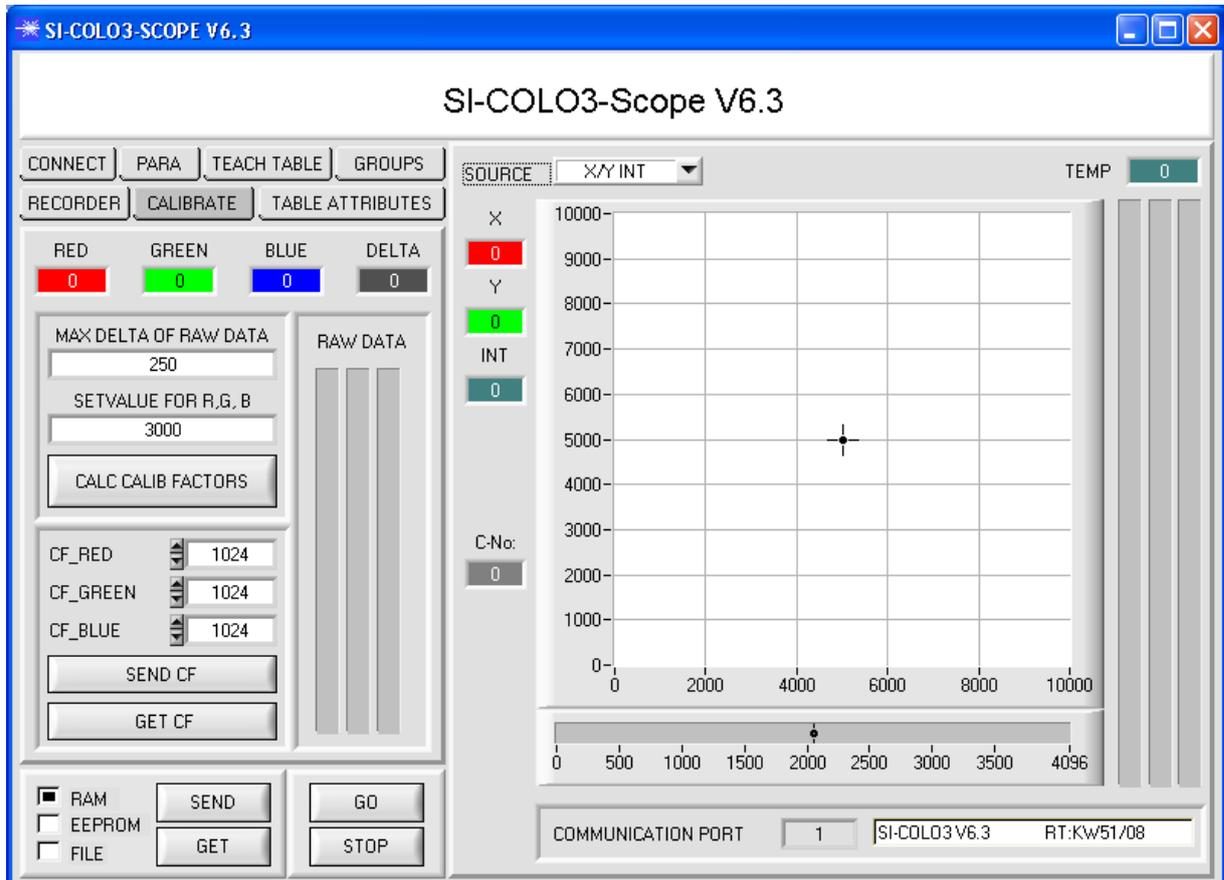
Calculation example for determining the calibration factors
