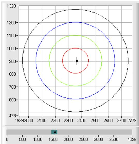
**Tip!** This mode is used if only one color is taught, and this color must be checked to avoid "drifting away". With the rising tolerance windows this can be detected very well, and countermeasures can be initiated, if necessary.
