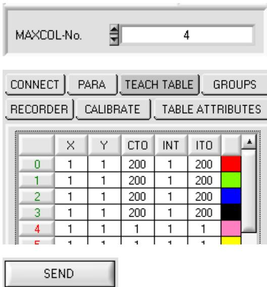
In this example, MAXCOL-No. = 4 was selected, i.e. the sensor should detect the color information that is stored in the first 4 rows of the TEACH TABLE by means of external teaching through IN0. Since the sensor cannot calculate the tolerances for color circle (CTO) and intensity (ITO) itself, these values must be entered once only (in this case 200 at all places) and must be stored in the EEPROM (see above) together with the MAXCOL-No. and with EXTEACH = ON.
