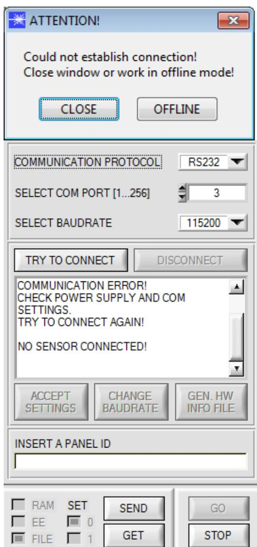
If a connection is not established automatically, e.g. if no sensor is connected, the software can be run in OFFLINE mode. In offline mode it only is possible to exchange parameters with a file on a storage medium, which often is helpful for the purpose of analysing parameter files.
