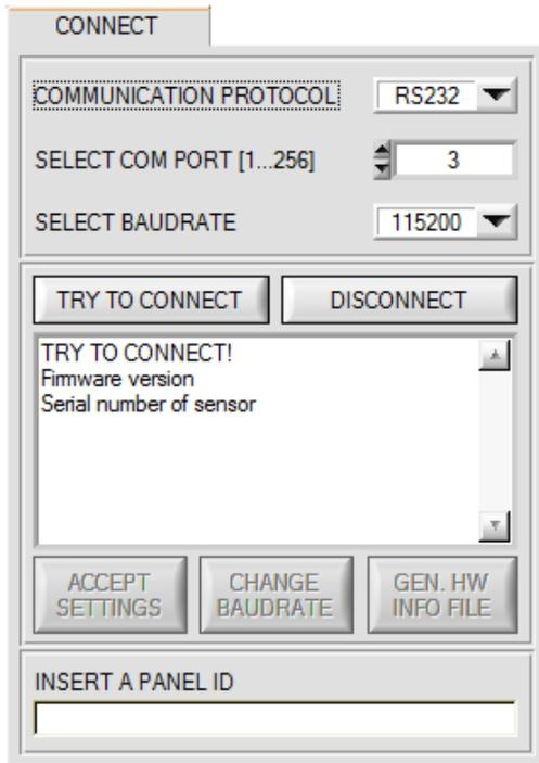
1. When a connection is established the serial number of the contacted sensor is transferred in addition to the firmware version.
