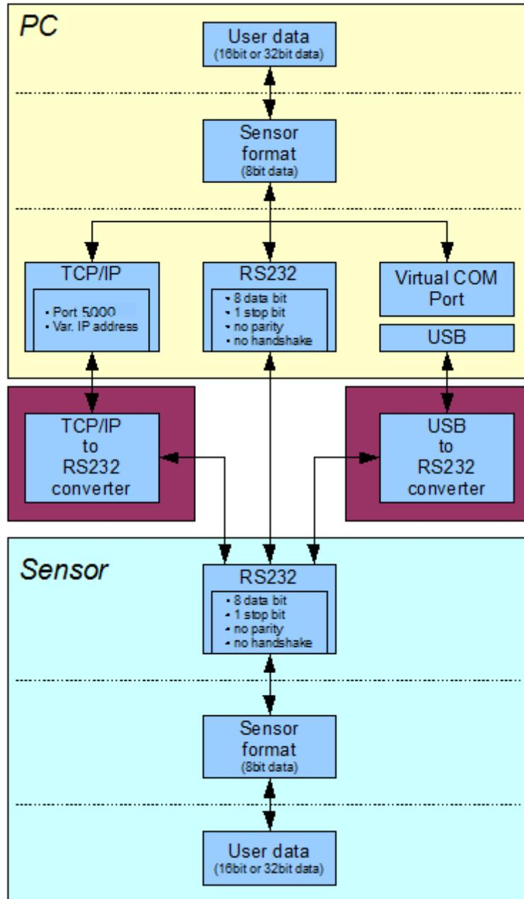
A proprietary protocol format that organises and bundles the desired data is used for all physical connection variants between PC software and control unit. Depending on their type and function the actual data are 16- or 32-bit variables and represent integer or floating-point values. The protocol format consists of 8-bit wide unsigned words ("bytes"). The actual data therefore sometimes must be distributed to several bytes.
