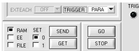
On the software interface the status of IN0 is displayed by the **TRIG** LED. If this LED is black, IN0=LO=0V, and the sensor operates with parameter set 0.
