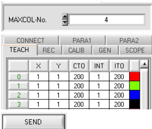
In this example, **MAXCOL-No. = 4** was selected, i.e. the sensor should detect the color information that is stored in the first 4 rows of the **TEACH TABLE** by means of external teaching through IN0. Since the sensor cannot calculate the tolerances for color circle (**CTO**) and intensity (**ITO**) itself, these values must be entered once only (in this case 200 at all places) and must be stored in the **EEPROM** together with the **MAXCOL-No.** and with **EXTEACH = ON**.
