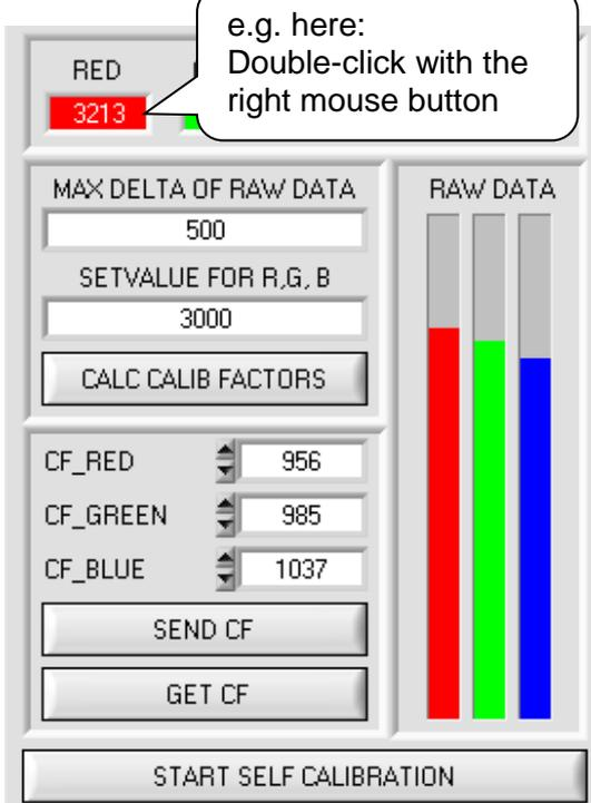
Offset calibration can be accessed by double-clicking with the right mouse button at any place between the individual elements in the **CALIBRATE** tab.
