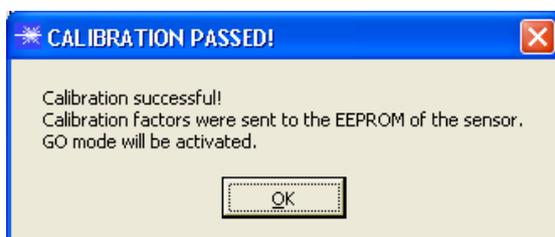
A click on **START SELF CALIBRATION** causes the sensor to calculate the calibration factors itself. It is not possible to specify a **SETVALUE** and a **MAX DELTA** here.
