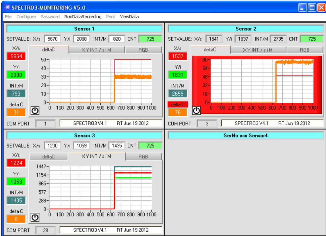
The data that are selected in the **OUTPUT FILE CONFIGURATION PANEL** are immediately saved in the correspondingly created file, if this is activated, and are visualised on the screen. The **CNT** display shows the total number of recorded values.
