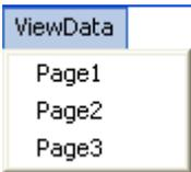
For reasons of space only 4 sensors can be displayed on a screen. **"Page1"** and **"Page2"** can be used to toggle between the first 4 and the last 4 sensors. **"Page3"**, however, displays the delta C and the C-No. of all 8 connected sensors.
