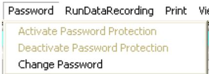
The **"File"** and **"Configure"** items can be protected by a password. Password protection can be enabled and disabled. The default password is: 0000000000 (in words: 10 zeros). The password can be individually changed.
