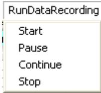
In this menu item data recording can be started with **"Start"** and stopped with **"Stop"**. Data recording furthermore can be paused with **"Pause"** and then continue again with **"Continue"**.
