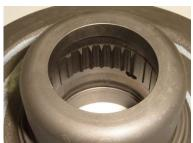
is around 93mm. The internal geared wheel must be turned during the movement and the relation between the teeth and the gap length informs about a good or a bad internal toothing.
