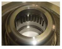
the distance to the teeth is around 93mm. The internal geared wheel must be turned during the movement and the relation between the teeth and the gap length informs about a good or a bad internal toothing.
