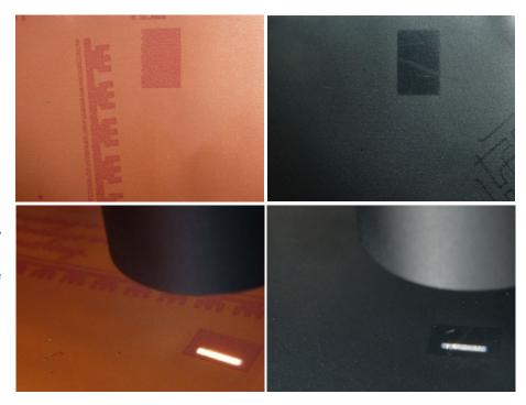
at the color mark distance is around 4mm x 0.7mm. In selecting the color mode **THD** in addition to **EXT TEACH ON** the color marks can be proper detected as shown in the screen shots.
