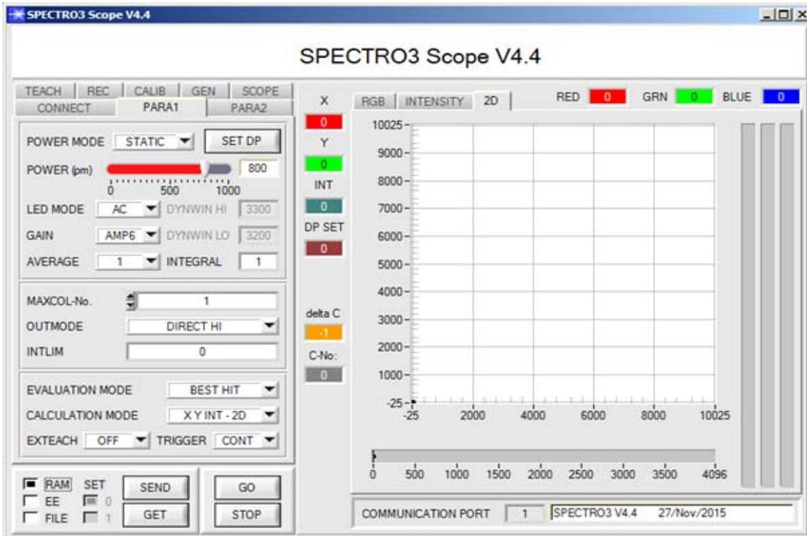
Under Windows® representation of the color value on a PC in numeric form and in a color chart, and representation of RGB values in a time chart. In addition the current RGB values are displayed as a bar chart.
