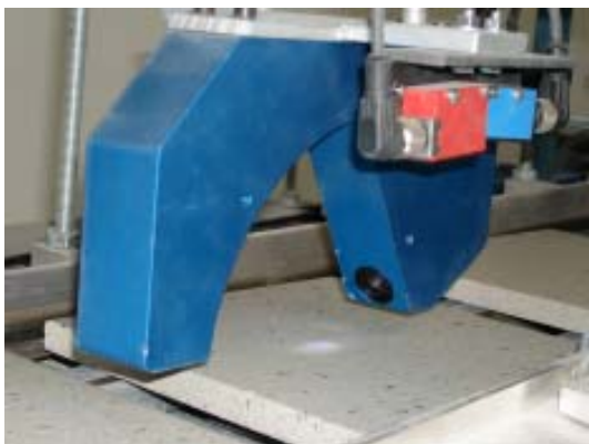
Gloss degree monitoring at plates of stone
