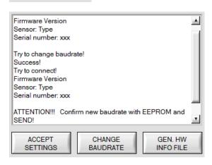
When the new baudrate information has been successfully sent, the sensor operates with the new baudrate. A window will pop up, prompting you to select **EEPROM** and then to press **SEND**. After a hardware reset the new baudrate only will be used when **EEPROM** and **SEND** have been pressed.
