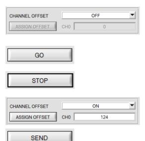
To determine the current offset, first work with **CHANNEL OFFSET = OFF**.
