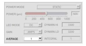
With CHANNEL OFFSET = ON certain setting possibilities that may influence the offset are grayed out. If you wish to change such settings you must first select CHANNEL OFFSET = OFF, then make the respective settings, and finally determine the offset anew.
