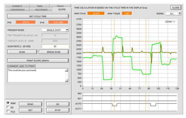
The zoom function in the graph can be activated by holding the control key (CTRL) and drawing a window with the mouse.
