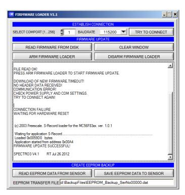
INFO! In case that the sensor was "killed", the sensor will work with a BAUDRATE of 115200.
