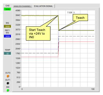
After a positive signal (+24V) at input IN0 the transmitter power is adjusted such that the sensor is in its dynamic range, which is set by **DYN WIN LO** and **DYN WIN HI**.
