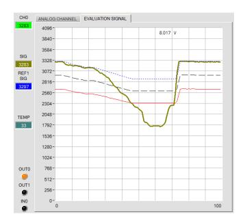
In this example a value of 50 was specified for **TT DOWN**. This means that downward threshold tracing is performed at a relatively slow speed.
